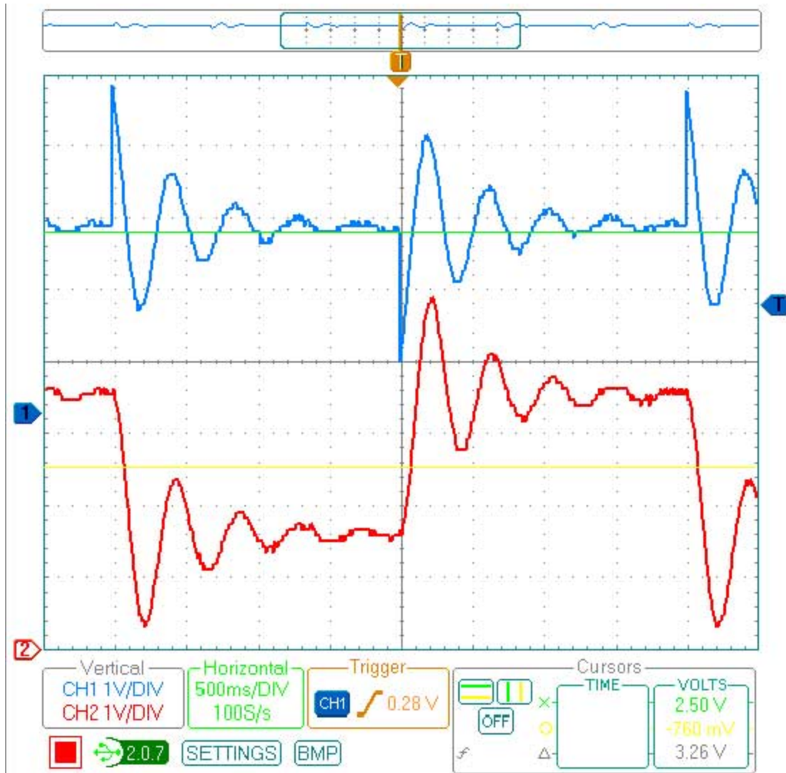
Figure 4.0 Input and Output Waveforms for a Working Digital Lead Compensation Network
