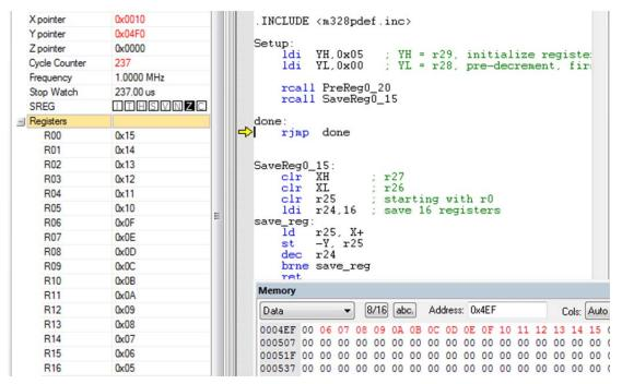
Figure 2 Registers r0 to r20 saved to stack buffer starting at location 0x04FF.
