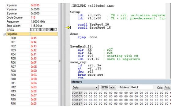
Figure 1 Registers r0 to r20 preset to values 0x15 to 0x01.
