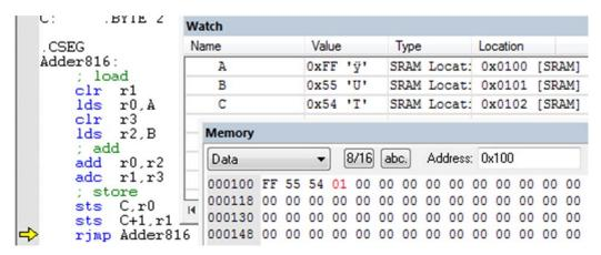
Figure 2 End of Addition program with variable C containing 0x0154 ( $340_{10}$ ). Byte ordering is little endian.
