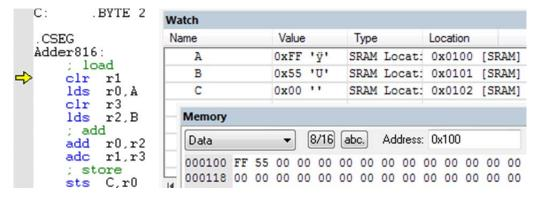
Figure 1 Start of 8-bit Addition program with variable A initialized to 0xFF (255<sub>10</sub> unsigned) and B initialized to 0x55 (85<sub>10</sub> signed).
