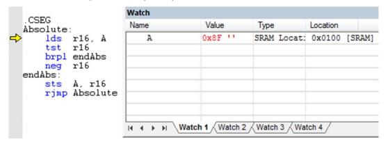
Figure 1 Start of Absolute program with variable A initialized to  $-71_{16}$  (-113<sub>10</sub>)
