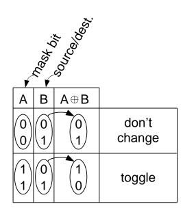
When toggling an I/O-Port bit, consider writing a one to the corresponding pin.
