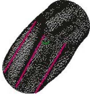
Buckling pattern of a thin-walled tube under torsion.
