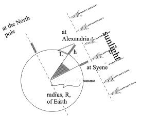
Vertical objects are located at various latitudes. The shadow cast by each can be obtained by using a line parallel to the incoming rays of the sun. Draw the line from the top of the object toward the horizon plane of the object.
