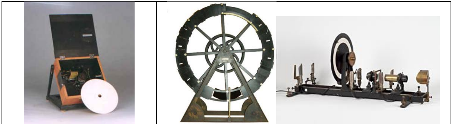
(Left) To study memory Hungarian psychologist Pál (Paul) Ranschburg developed “The Ranschburg Memory Device” in the early 1900s. The device consists of a box containing a rotating disk visible through a slot in the top. Experimenters can use the box to visually present a successive series of stimuli such as letters, words, numbers, symbols etc. at a controlled rate of presentation. The experimenter draws the stimuli on the disk and uses the box’s motor to control the rate of presentation of stimuli through the slot. From: University of Toronto (Right) The tachistoscope allows researchers to present images for a specific and controllable time period. The inventor of the tachistoscope remains unclear, though historians usually attribute the first general description of the device to the psychologist A.W. Volkmann in 1859. From: National Taiwan University and Recycled reads .
