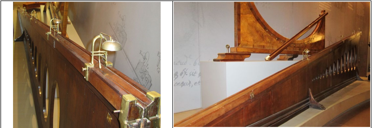
Pictures of the actual inclined plane apparatus used by Galileo to test the principle of universal gravitational acceleration and determine a value for g . Balls rolled down the tracks ringing bells to help with timing. The inclines could be changed in some cases to increase or decrease the vertical component force of g accelerating the balls. From: Arbor Scientific 126
