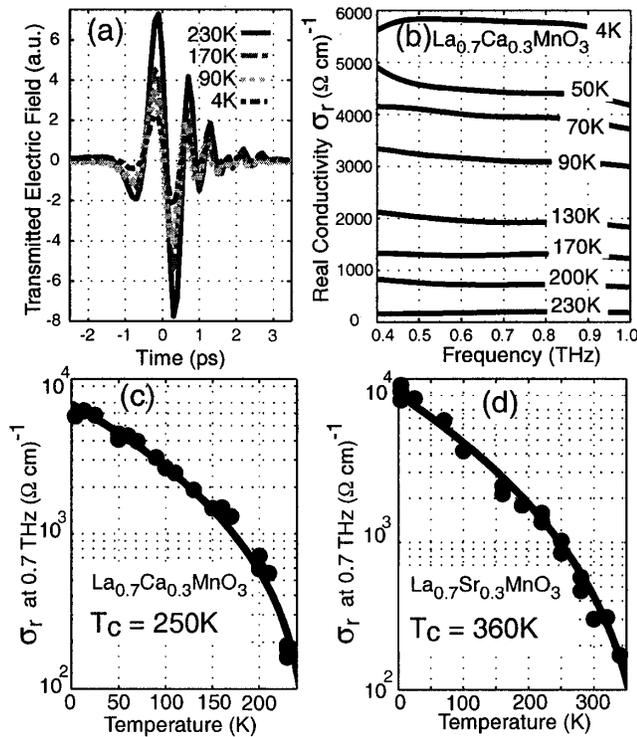
FIG. 1. Temperature dependence of the THz transmission and real conductivity. (a) Transmitted electric field at various temperatures for a 90-nm thick LCMO film. (b) Real conductivity versus frequency for LCMO at various temperatures. (c),(d) The value of the real conductivity at 0.7 THz as a function of temperature for LCMO and LSMO thin films. The lines are fits using Eq. (1).
