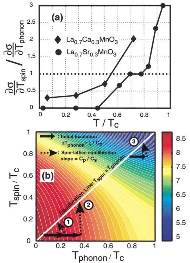
FIG. 4 (color). (a)  $\partial\sigma/\partial T_s$  divided by  $\partial\sigma/\partial T_p$  versus the initial temperature. The dots (lines to guide the eye) are experimental data. (b) Contours of constant conductivity are plotted in the  $T_p$ - $T_s$  plane [the color bar is  $\ln(\sigma)$ ]. The curved white lines highlight the contours of constant conductivity. The arrows labeled 1 to 3 are discussed in the text.
