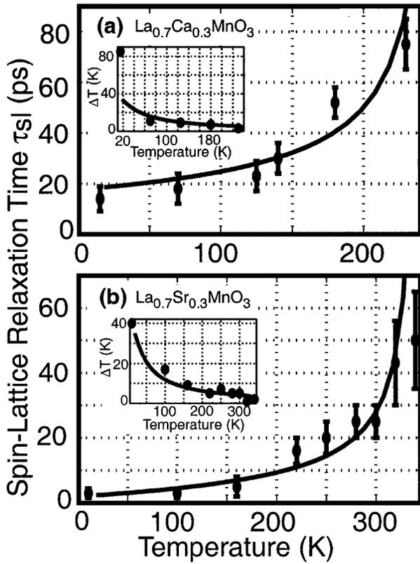
FIG. 3. (a),(b) Temperature dependence of the lifetime  $\tau_{sl}$  of the slow component due to spin-lattice relaxation for LCMO and LSMO, respectively. The solid lines are fits as described in the text. The inset shows the induced temperature change as determined from the conductivity measurements (dots) and the calculations (solid line).
